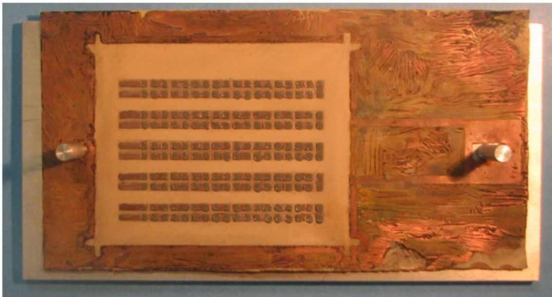
Figure 62: Bottom circuit board after successful solder paste application
