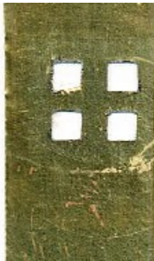
Figure 26: First etched sample – Brass trial solder stencil
