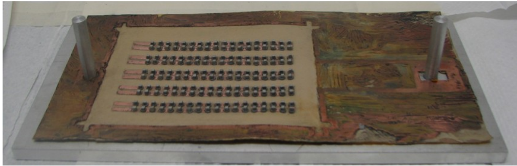
Figure 66: Remaining thermoelement templates removed after n-type thermoelements are positioned
