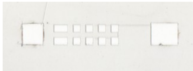
Figure 46: Transparency based solder stencil used on third and fourth trial assemblies
