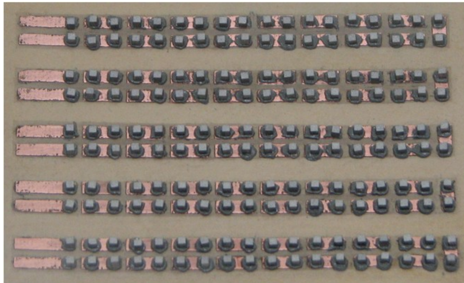
Figure 67: Close up of the thermoelements positioned on the bottom circuit board
